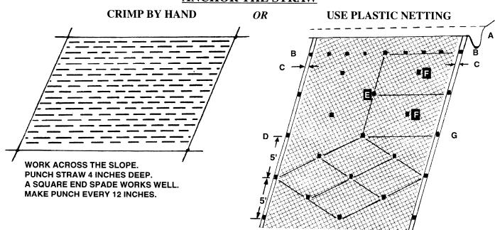
A. LAY BIRD CONTROL NETTING OR SIMILAR MATTING IN STRIPS DOWN THE SLOPE OVER THE STRAW. BURY UPPER END IN 6-8 INCH DEEP AND WIDE TRENCH.. MOST NETTING COMES IN 14 TO 17 FT. WIDE ROLLS.
